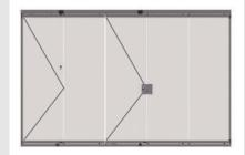
The Moving Door can be placed in any part of the **Seeglass** system and it can be opened and closed according to the client's needs without having to open the entire system.
