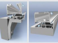
This new auxiliary condensation profile is specially designed to drain out the water that forms due to temperature changes. It can be installed with or without bracket support.
