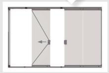
The moving door functions as another panel which slides and folds to the side when the system is open.
