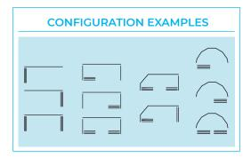
Seeglass systems let you slide glass panels in any way desired, being able to adjust to almost any possible configuration. Openings can be internal or external, and have opening devices on the inside or outside. Additionally, all the panels can be easily cleaned.
