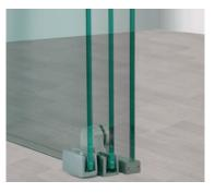
Portavant 60 twinline, the twin-track Portavant solution for a wider clearance width, combines a synchronised telescopic function with a cushioning and self-closing system on both sides of the sashes, while requiring a profile height of only 70 mm.
