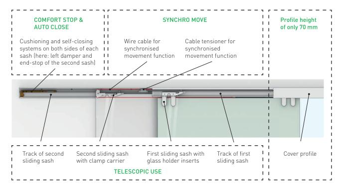
Portavant 60 twinline is a true miracle in the compact use of space. Despite telescopic technology, synchronised movement and a cushioning and self-closing system on both sides of each sash, it only requires a profile height of 70 mm. And with 10 mm glass thickness, for example, it requires a distance of less than 25 mm both between the two sliding sashes and between the second sliding sash and the wall or sidelight.
