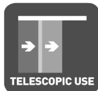
**TELESCOPIC USE** The telescopic solution for a wider clearance width: ensures that the sliding sashes require very little room when they are open.
